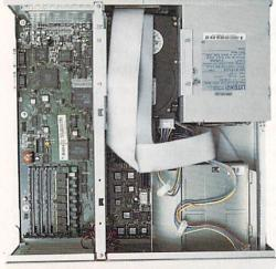
The A4000 is designed for easy access to install hard disks, RAM, and CPU cards.
